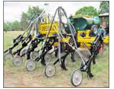
The Pasture Kropper plants direct into existing pastures. CONTRIBUTED
